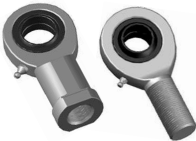
Rod ends EXHI..DO (2RS), EXHE..DO (2RS) Steel/Steel made up of a radial spherical plain bearing BJ..E or BJ..E 2RS and rod body, with right or left-hand & male or female thread.
